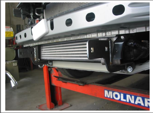
Figure 9: ECB steel mounting brackets fitted.
