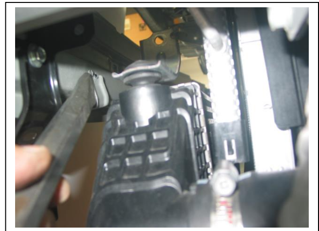
Figure 6: Chisel off temp sensor mount
