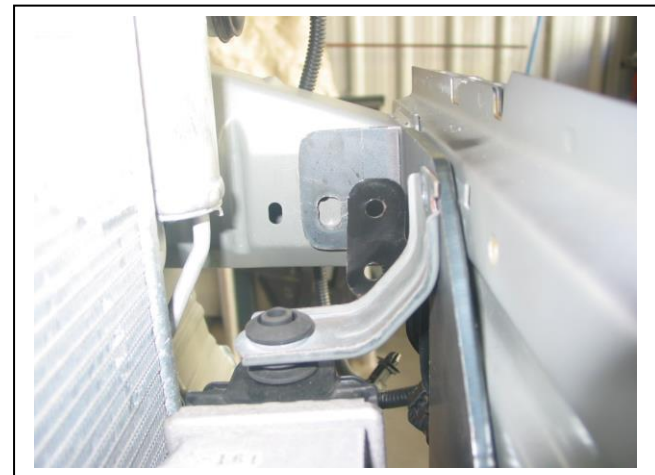
Figure 8: Flattened tab on top intercooler mount
