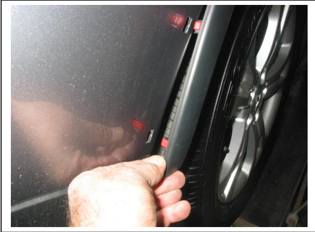
Figure 3: Removing wheel arch flair.
