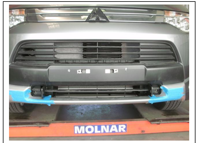
Figure 12: ECB steel mounting brackets with bumper fitted.
