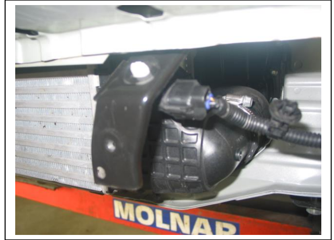
Figure 10: Temperature sensor on bumper locator.
