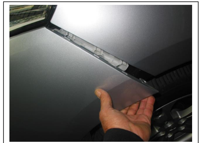
Figure 2: Carefully remove bumper from guard clips
